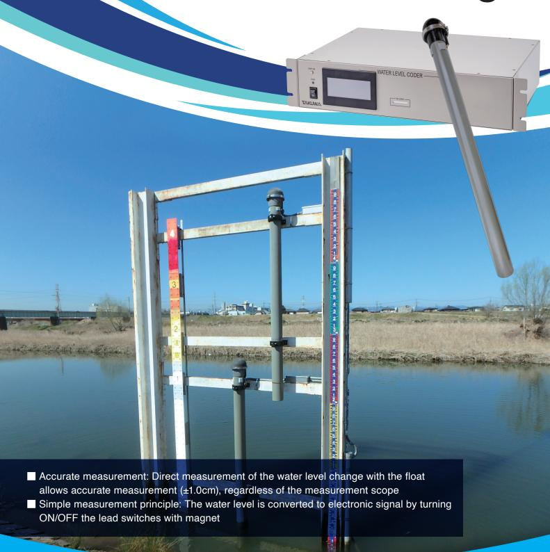
This product has a number of reed switches vertically at 1cm intervals. The float with a built-in permanent magnet moves up and down according to change in the water level, and it turns on the switch at a level in the gauge to sense the water level.
