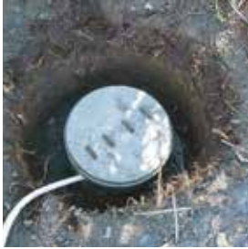
Vibration sensor (underground installation using hand hall)
